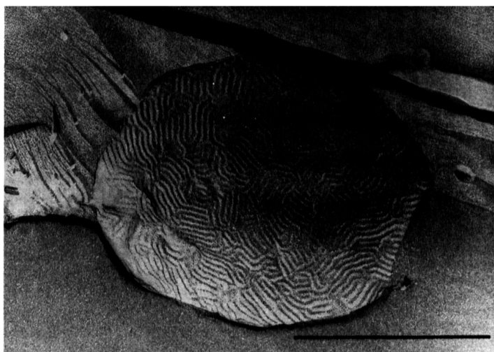
Fig. 2. Freeze-fracture electron micrograph of a vesicle composed of DMPC and DMPG (1:1) showing the typical 'ripple phase' (P B ) on the vesicle surface (freeze-fracture temperature: 17^\circ\text{C} . Magnification \times 46000 ).
